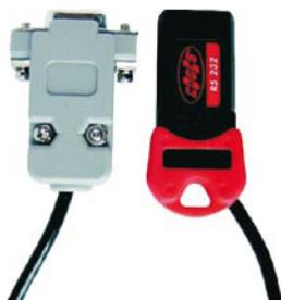
**(GB)** A key used to transfer data stored in the E.C.S. system directly to the portable PC, palm-top computer or printer, using the RS232 serial line.
